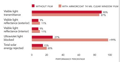
All performance results are based on the film installed on the inside surface of 4mm and 4mm+4mm thick, clear glass.
